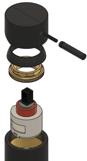
**PLEASE NOTE:** The cartridge can only be changed without water pressure! Do not open the tap until the water supply to the tap is interrupted in order to avoid damage to property and personal injury. When changing the cartridge, make sure that the contact surface of the cartridge seal in the body of the tap is free of dirt, traces of corrosion and/or other foreign bodies.
